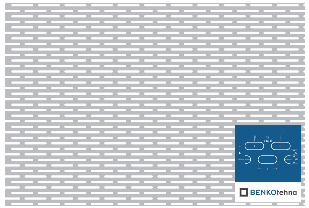
**Podolgovata zamaknjena Pz 2×20 - 5×24:** w = 2,0 mm |  $c_1$  = 3,0 mm |  $c_2$  = 4,0 mm |  $t_1$  = 5,0 mm |  $t_2$  = 24,0 mm | I = 20,0 mm | **odprtost** = 32,62%
